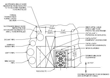
\* ABSOLUTE MINIMUM CLEARANCE 0'-9" AT LOCATIONS WITH REDUCED WIDTH SHOWN ON DWGS PER-E-C-964 TO PER-E-C-969
